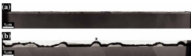
Fig. 6 Montages of the cross-sectional TEM images of films heat treated at a 1300 °C for 1 h, b 1400 °C for 1 h. The dark layer is the Pt coating used to protect the original surface during FIB preparation
